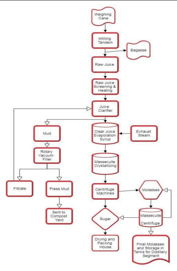
The output from the above process is then inserted in the Multiple Effect Evaporation System which results in Syrup like substance and stored in Syrup supply tanks. The Syrup in the Syrup supply tank is then subjected to the process of Crystallizing and Massecuite in various centrifuge machines giving us sugar crystals.
